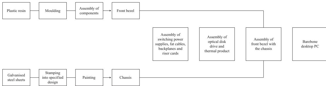
The production process for PC enclosures involves the production of chassis and final assembly. Components and peripherals are assembled into various types of enclosures according to customers' specifications. The Company manufactures the chassis, connectors and cable assemblies, flat cables, thermal products, backplanes and riser cards used in the manufacture of enclosures and purchases the remaining components and peripherals from third party suppliers.
